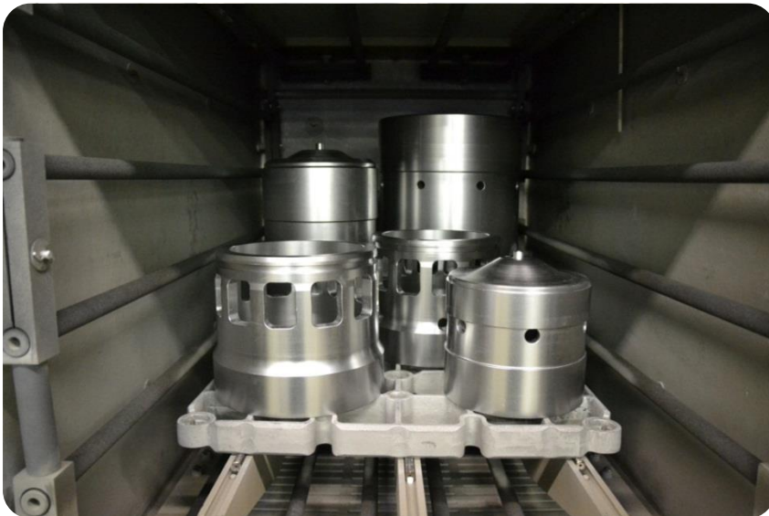
Heat chamber of the SCHMETZ vacuum hardening furnace
