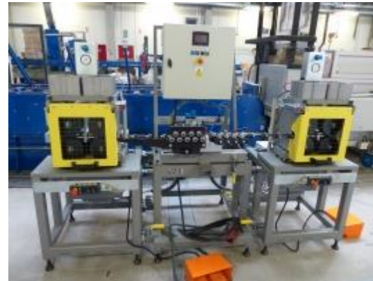
Universal straightening line for wires and tubes
