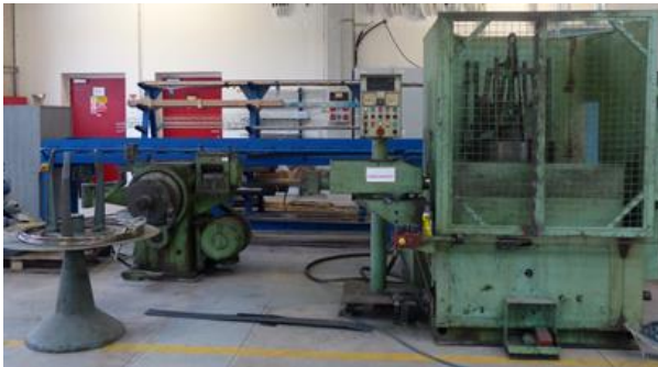
Precise drawing line for diameters 15-0.2 mm
